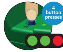
**STEP 1:** Press the reset button 4 times.
