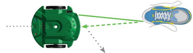
The S3's rear tail wheel is a stall sensor. If it get stalled on an object it cannot see, it will back up, turn, and try driving forward again.
