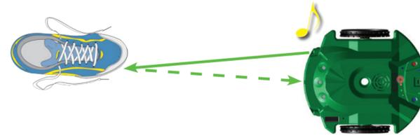
**EXTRA:** If the S3 can see the object with both sensors it will play both tones and both green LEDs will turn on. The S3 can usually see light objects better than very dark objects, because dark objects often do not reflect much infrared light.
