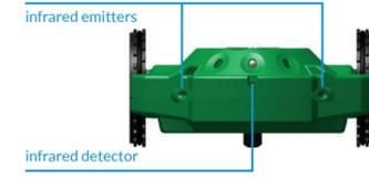
Infrared light shines from the emitters, even though your eyes cannot see it. The S3 robot can detect the light after it reflects off an obstacle and bounces back to its infrared detector "eye."
