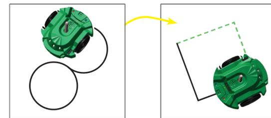
**NOTE:** Just like handwriting, each S3 drawing will be recognizable but unique every time you run a program. Variations occur as battery charge changes, motors warm up, and wheel joints relax with use over time.
