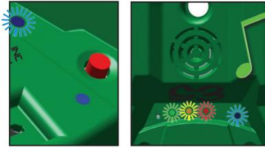
**STEP 3:** Cover a light sensor with your finger. An LED will turn off.
