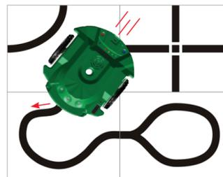
**EXTRA:** The S3 does best following black lines about 3/4 inch (2 cm) wide, on a white background. Line following works best when the track is placed on a hard, level surface. Carpet, tile, or other uneven surfaces may not work well. A dark surface may show through thin paper and make the line harder for the S3 to see.
